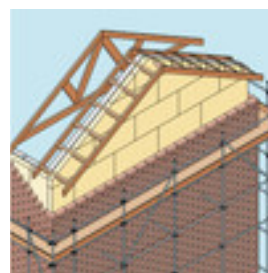
Figure 6. Installation of Batts in gable end wall
